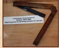
When viewing the Lyle Gun, be sure to notice the also newly acquired octant that has been placed in the exhibit just next to the Lyle gun. This beautiful piece of equipment was manufactured by The Chapin-Stephens Company in Riverton, Connecticut, circa 1900. It is made of boxwood and brass, and includes a metal fold-out scale and a bubble level. The gunner used the octant to set the firing elevation of the Lyle gun.
