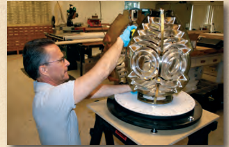
THE LENS IS INSTALLED ON THE ROTATING TEST PLATFORM
