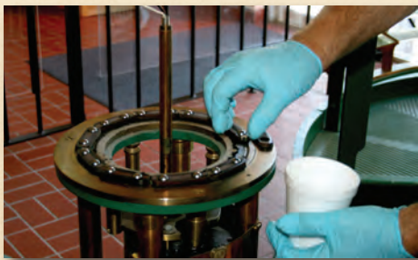
AFTER THE LAMP AND LENS ARE REMOVED THE ROTATION MECHANISM'S BEARINGS GO NEXT
