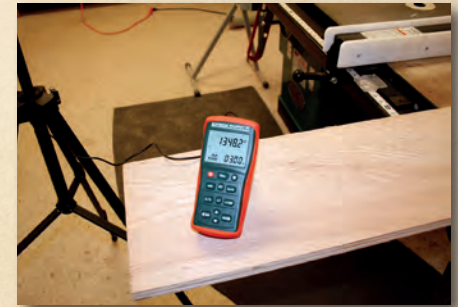
THE INTENSITY OF THE LIGHT EMITTED BY EACH PANEL IS MEASURED WITH AN ELECTRONIC LIGHT METER
