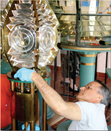
DAN SPINELLA PREPARES THE REPRODUCTION 6TH ORDER LENS FOR DISASSEMBLY
