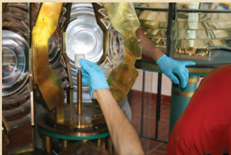
THE LAMP IS REMOVED FROM THE CENTER OF THE 6TH ORDER REPRODUCTION LENS
