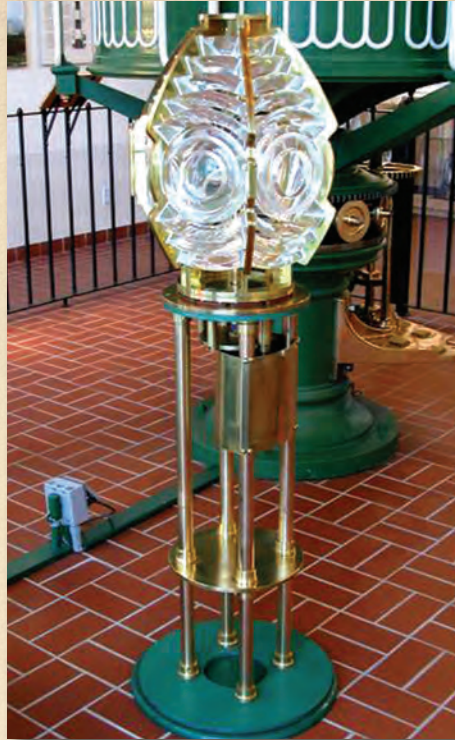
PONCE INLET LIGHTHOUSE'S REPRODUCTION 6TH ORDER ROTATING FRESNEL LENS
